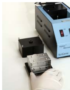
1. Place arrays in racks.
