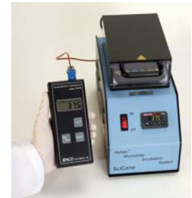
Calibration with a digital thermometer ensures accurate temperatures.
